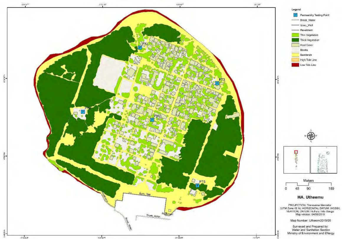
Figure 3.14: Locations of permeability tests in Utheemu Island
