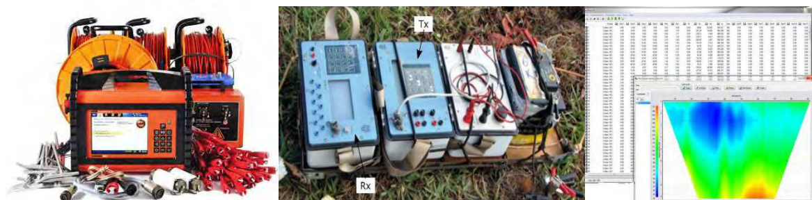
Figure 1.4. Electrical Resistivity (ER) equipment used for the field pilot tests
