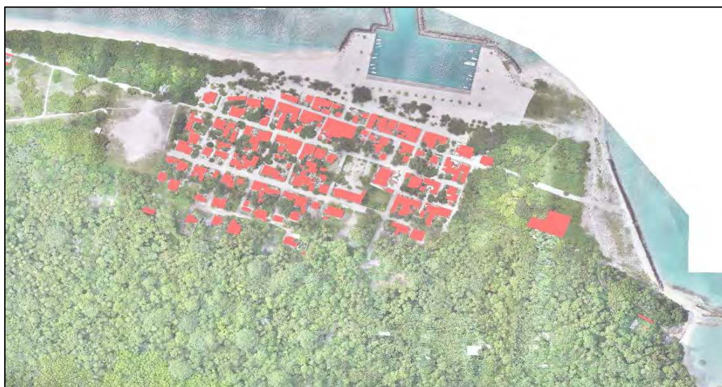
Figure 1.6 – Calculation of Roof Cover in an island using UAV survey in Maldives
