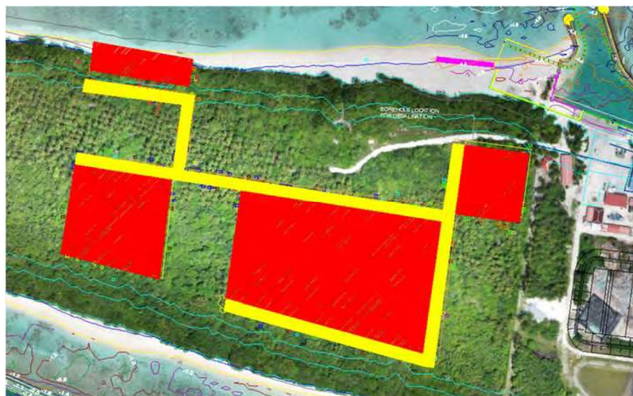
Figure 33. Areas which require vegetation clearance to develop the plots (red) and roads (yellow) as per the proposed master plan
