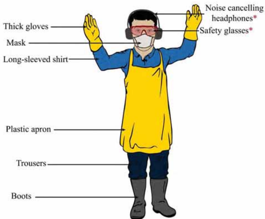
Figure 23: Recommended protective clothing for waste management employees. Adapted From: Ministry of Health, Thailand. Bangkok, 1995. *noise cancelling headphones and safety glasses during use of machinery
