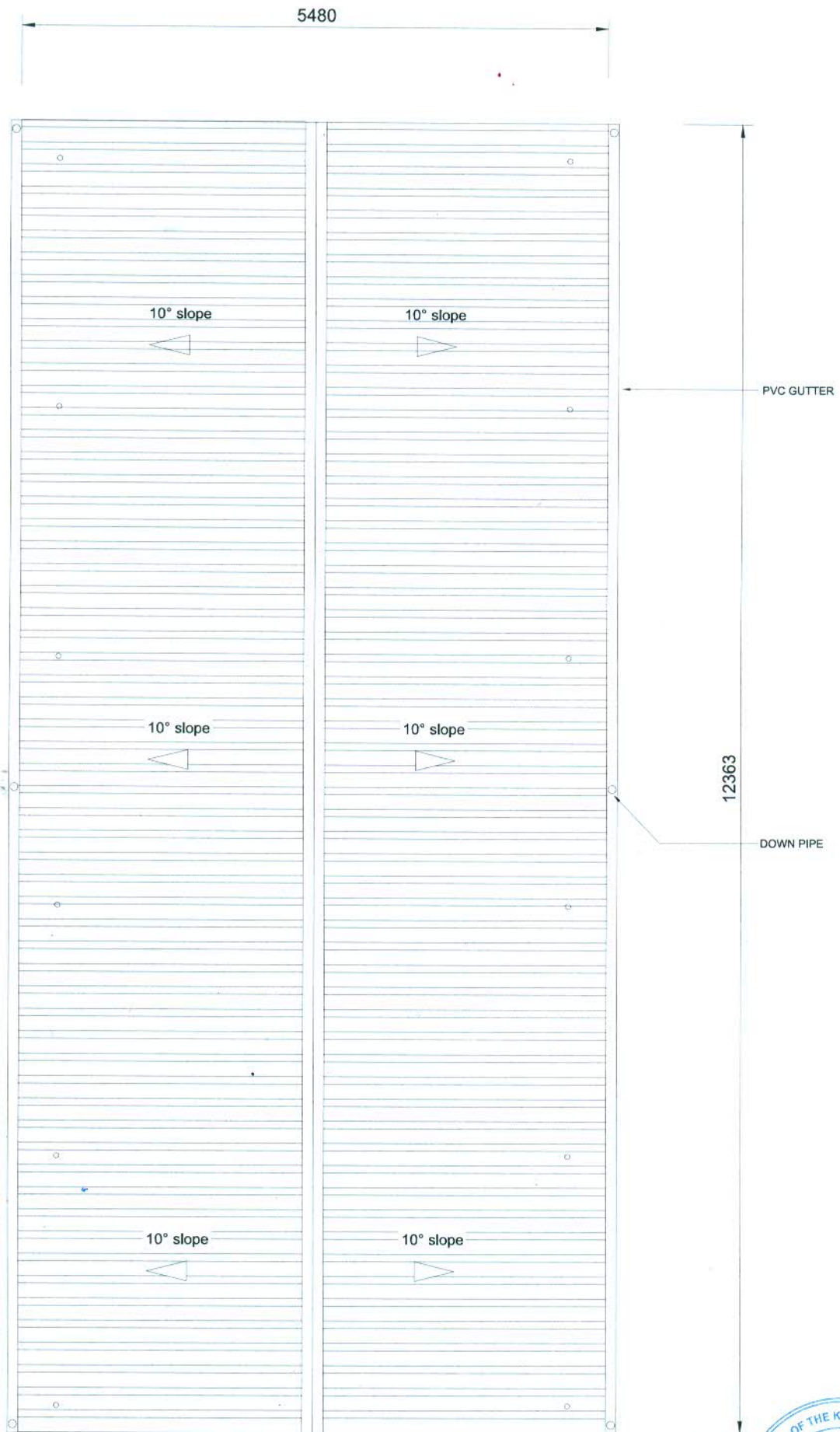
ROOF PLAN OVER WATER TANKS COUNCIL SITE
