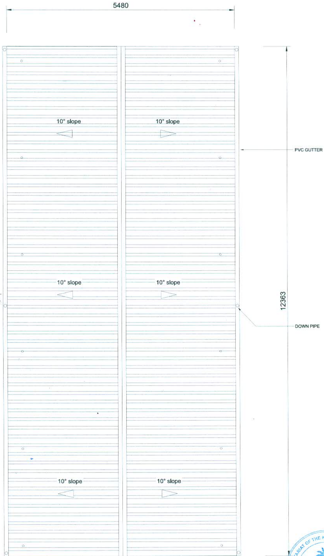
ROOF PLAN OVER WATER TANKS MASJID-UL THAQVAA
