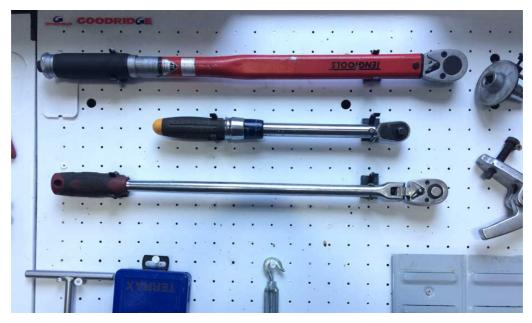
A torque wrench is a tool that tightens fasteners to an adjustable specific measurement. All nuts, bolts and screws will have an exact torque specification, set out by the manufacturer.
