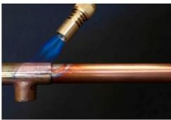
The melting point of parent metal should be higher than
