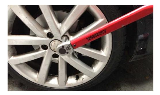
A torque wrench is also needed when replacing a water pump, front engine cover, camshaft cover, oil pan etc. Over-tightening these components can lead to oil leaks and serous engine damage.
