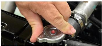
Check the coolant level during shutdown periods at the specified interval. Remove the radiator cap after allowing the engine to cool, and, if necessary, add coolant until the level is about 3/4 in. Heavy-duty diesel engines require a balanced coolant mixture of water, antifreeze, and
