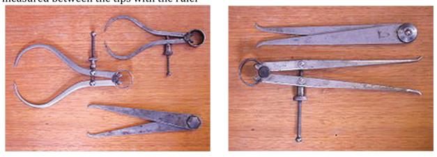
Fig. 4.3: Outside callipersFig. 4.4: Inside callipers
