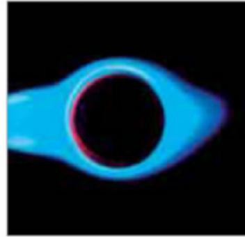
Soft Soldering central heating pipe Flame beating action on joint
