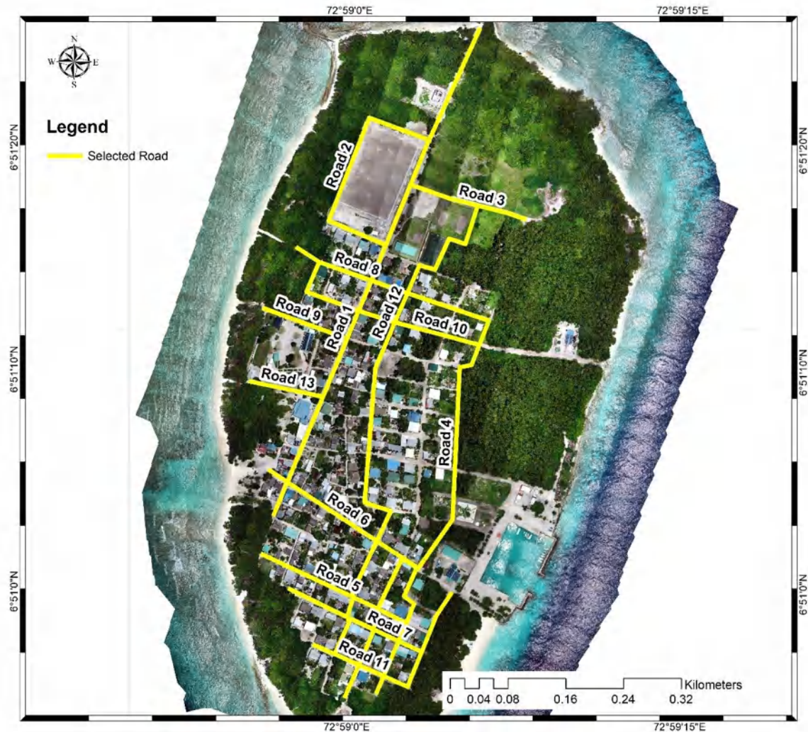
Figure 4–4: Selected Roads for Recharging trenches and pits
