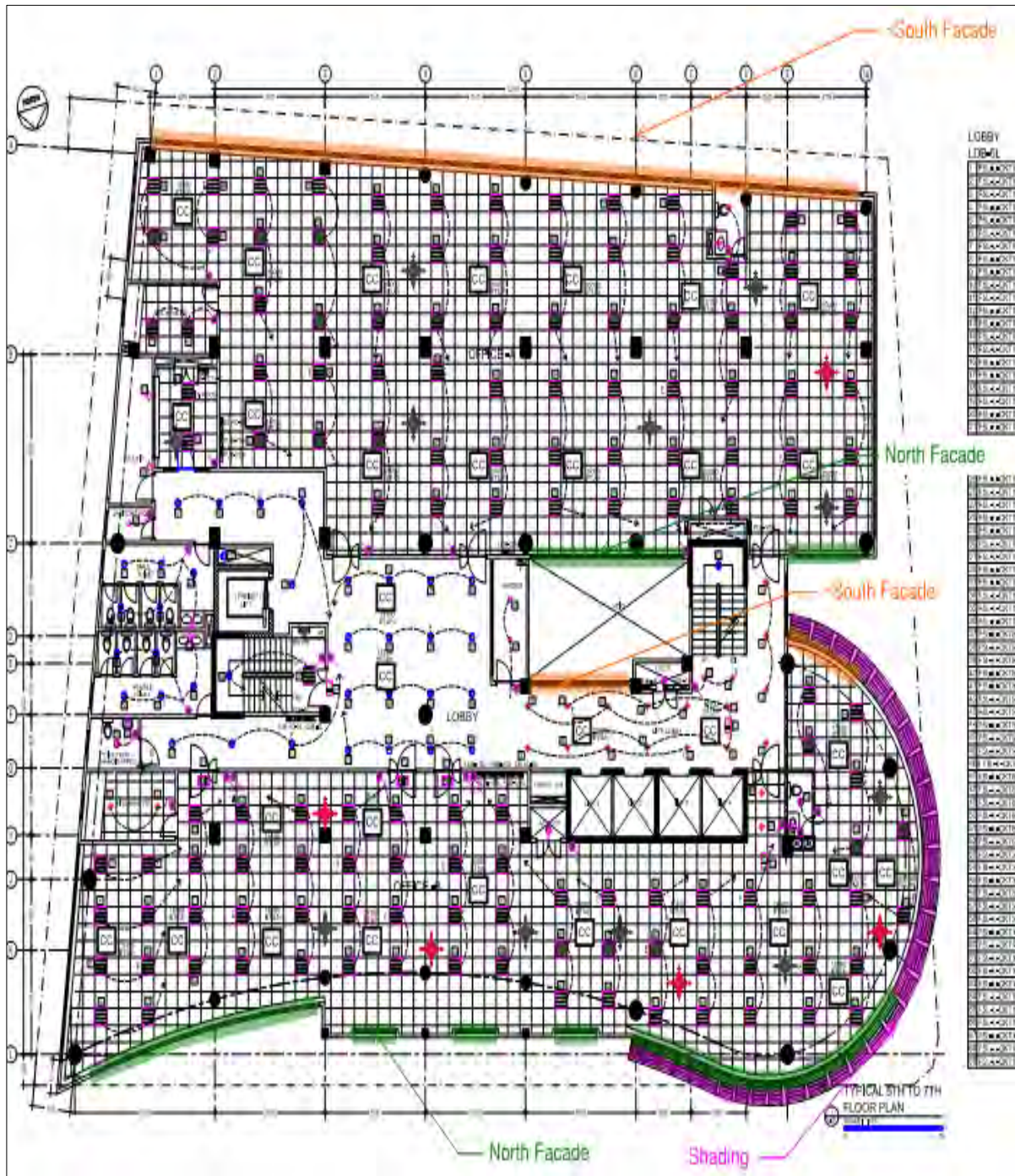
Figure 1-26: General building layout showing Image showing shading and relative proportion of north and south facades
