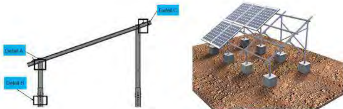
Figure 3-16: Installation of mounting structures
