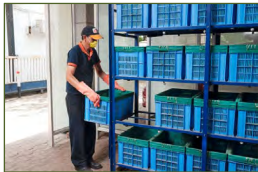
Pic 4: Place raw compost in the curing system for 10-day maturation cycle
