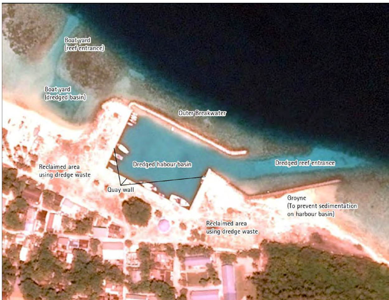
Figure 4.1 Basic elements of harbor infrastructure
